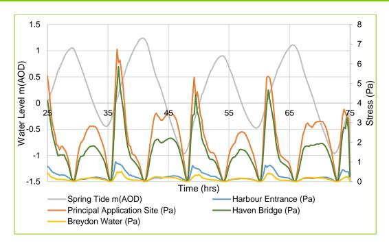
Plate 6-25: Model Predicted Scheme Bed Stress - Spring Tide
