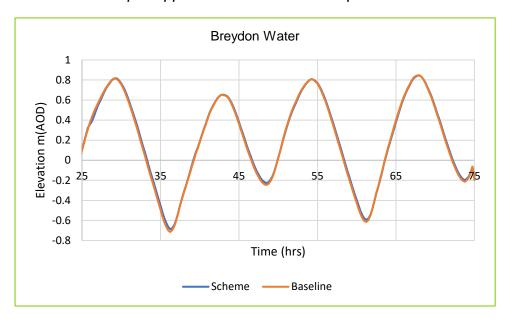
Plate 6-20: Comparison of Water Level between the Baseline and Scheme Scenarios at Breydon Water for the Neap Tide
