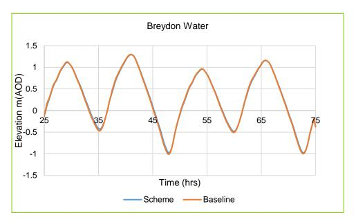
Plate 6-9: Comparison of Water Level between the Baseline and Scheme Scenarios at Breydon Water for the Spring Tide
