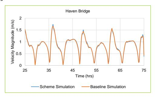
Plate 6-3: Comparison of Velocity Magnitude between the Baseline and Scheme Scenarios at Haven Bridge for the Spring Tide
