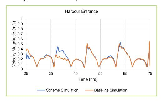
Plate 6-15: Comparison of Velocity Magnitude between the Baseline and Scheme Scenarios at the Harbour Entrance for the Neap Tide
