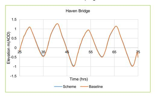
Plate 6-11: Comparison of Water Level between the Baseline and Scheme Scenarios at Haven Bridge for the Spring Tide
