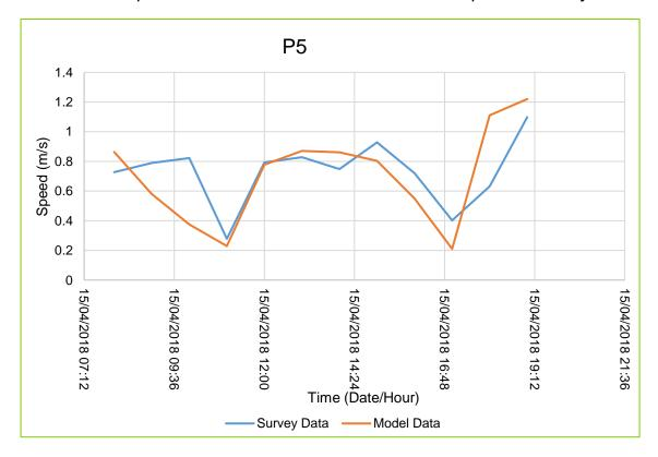
Plate 5-9: Comparison of Modelled and Recorded Water Speed at Survey Point 5
