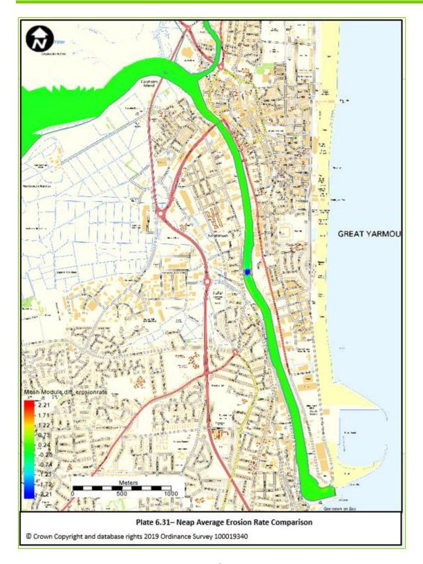
Plate 6-31: Neap Average Erosion Rate Comparison
