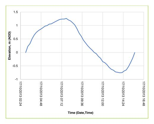
Plate 3.2: Typical Tidal Curve
