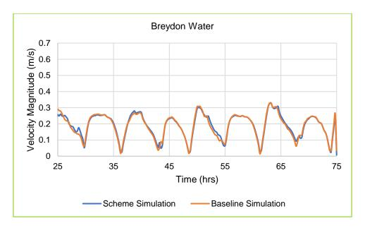
Plate 6-14: Comparison of Velocity Magnitude between the Baseline and Scheme Scenarios at Breydon Water for the Neap Tide
