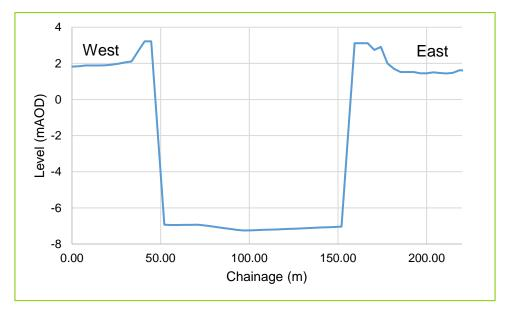
Plate 4-3: Typical River Cross Section: River Yare
