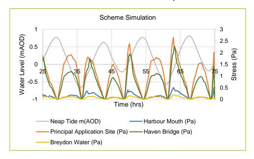
Plate 6-28: Model Predicted Scheme Bed Stress - Neap Tide
