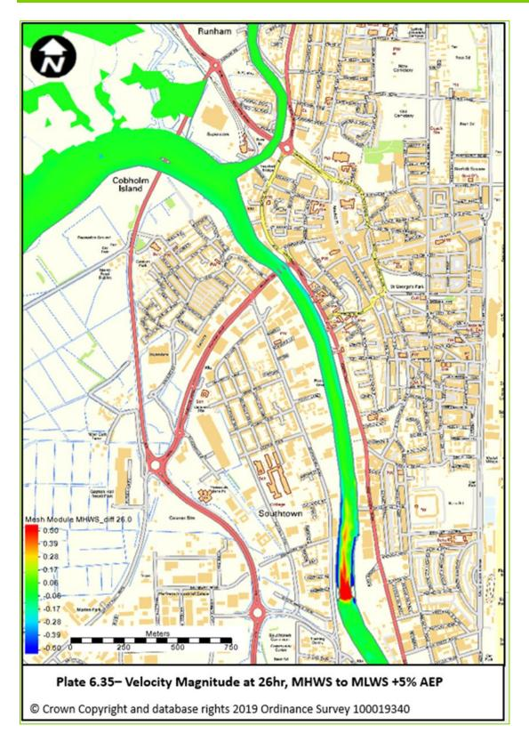
6.3.5 Plate 6-35 and Plate 6-36 show the velocity magnitude difference between the Baseline and Scheme scenarios in the MHWS-MLWS +5% AEP and MHWN-MLWN +5% AEP respectively. These figures show that velocity
