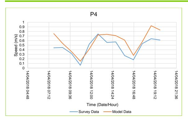
Plate 5-8: Comparison of Modelled and Recorded Water Speed at Survey Point 4
