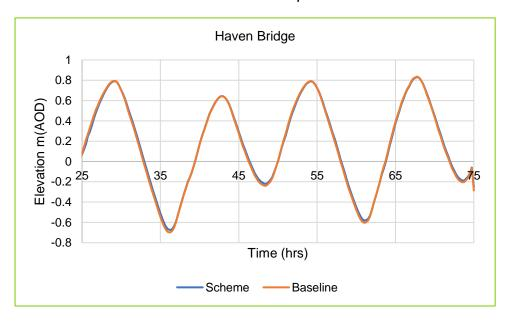
Plate 6-22: Comparison of Water Level between the Baseline and Scheme Scenarios at Haven Bridge for the Neap Tide
