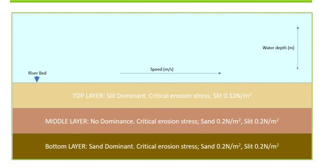
Plate 5-5: Sediment Model Layers Schematisation
